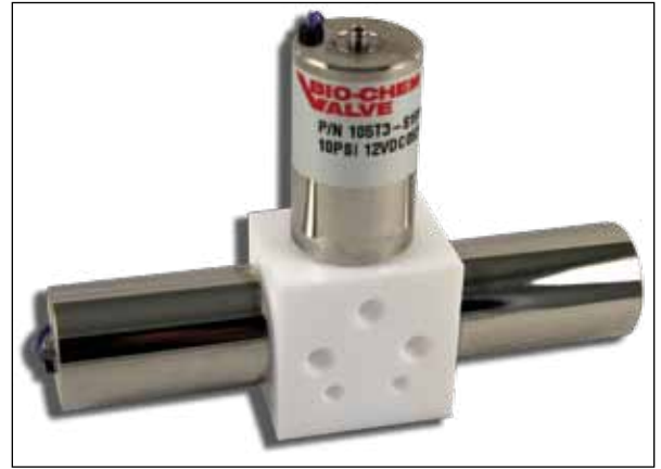
105T3 Flow Selection Valve (3 inlet ports, 0.125" orifice, PTFE body, PTFE diaphragm)
