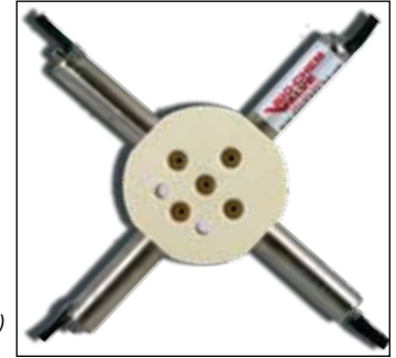
040T424-54-4E Flow Selection Valve (4 inlet ports, 0.054" orifice, PPS body, EPDM diaphragm)
